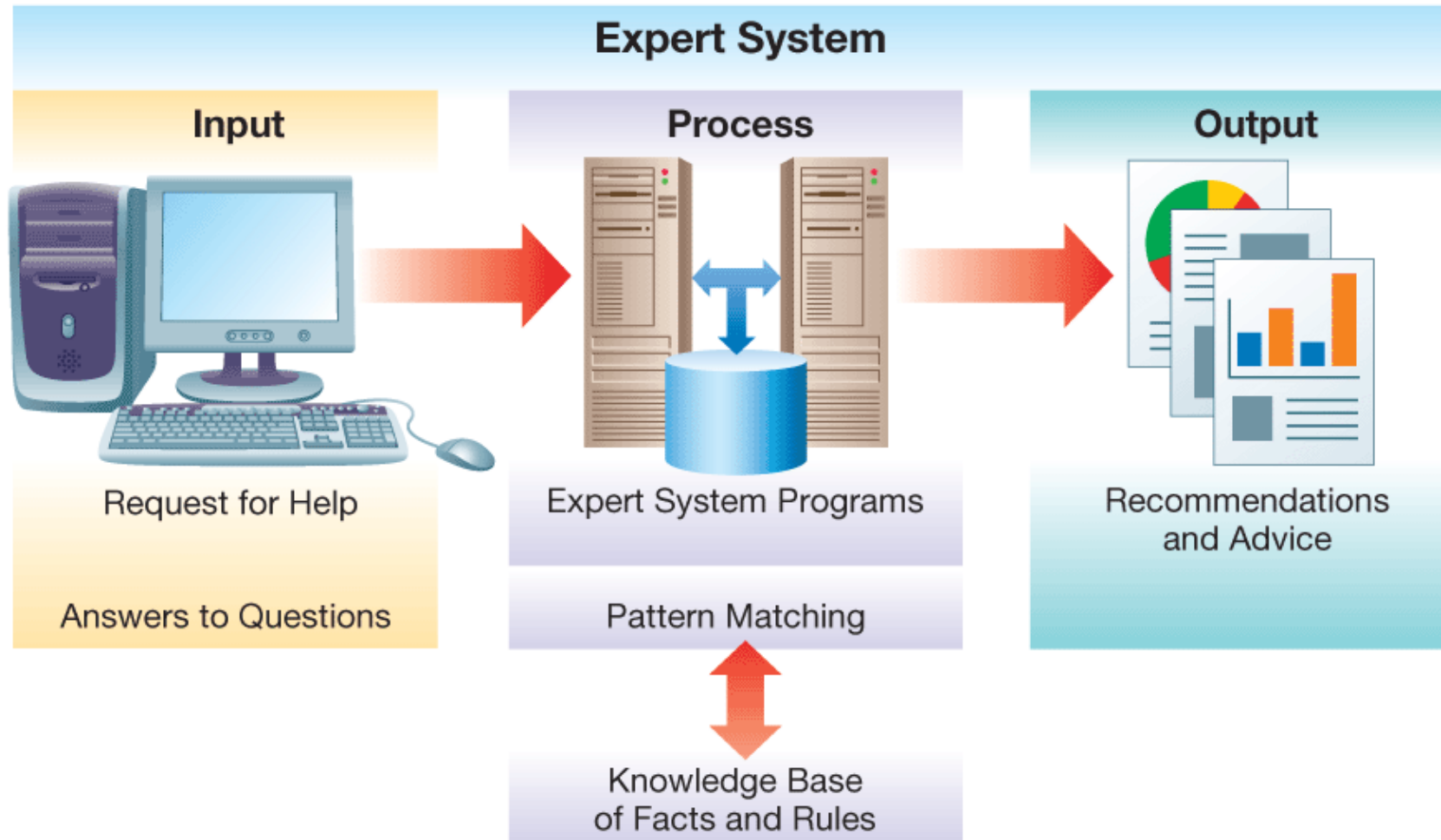
Figure 6.22 Architecture of an expert system using the basic systems model.
